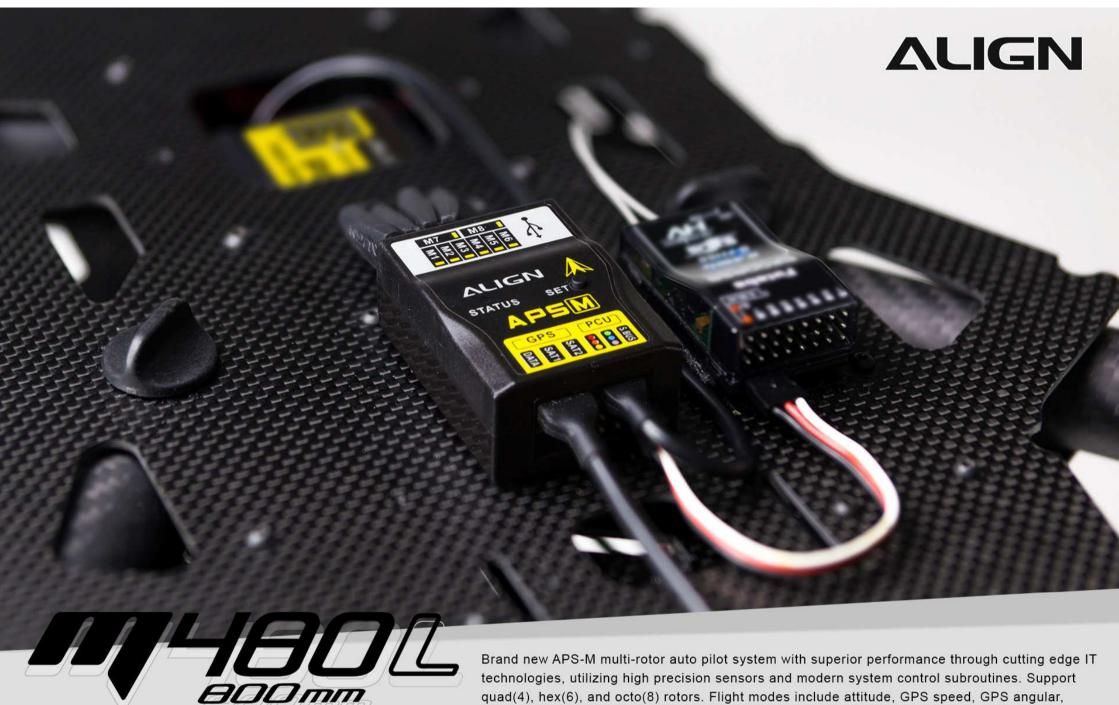
technologies, utilizing high precision sensors and modern system control subroutines. Support quad(4), hex(6), and octo(8) rotors. Flight modes include attitude, GPS speed, GPS angular, intelligent, and manual. In addition, it features GoHome failsafe, low voltage failsafe (through LED indicator and auto GoHome), OSD signal output, gimbal control, fix-point survey functions.
