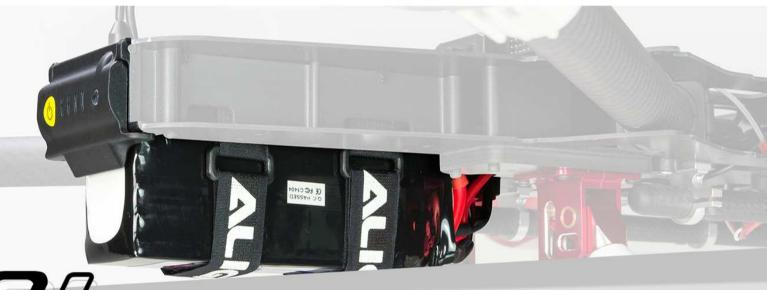
Quick release battery mounting plate and rail to allow for single handed quick battery replacement. Double decker battery mounting plate design to allow for single 6S (up to 12000mAh size dependent) battery, or two 6000mAh batteries. This system allows for flexible battery selection and variable CG adjustment.
